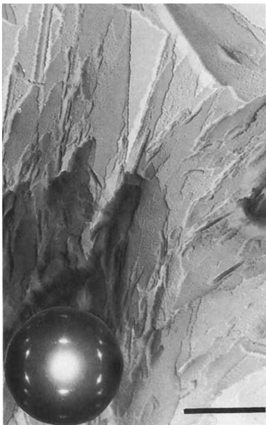
Figure 6 P-4-OB sample polymerized/crystallized 23 h at 270°C in a 1% biphenyl solution between glass (G/G). Inset shows the phase II hk0 orientation.
